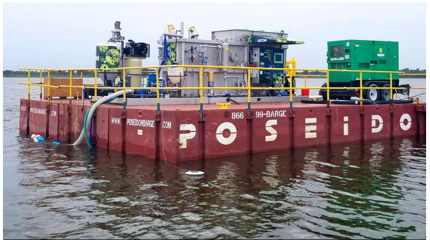
A harvesting unit mounted on a barge is being transported around Lake Jesup so that algae can be harvested at various locations .
